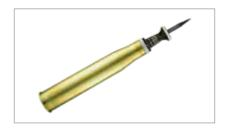
The projectile is crimped to the cartridge case which is loaded with cool burning, multi-perforated, loose propellant, and is fitted with a mechanical primer and a wear reducing liner.
